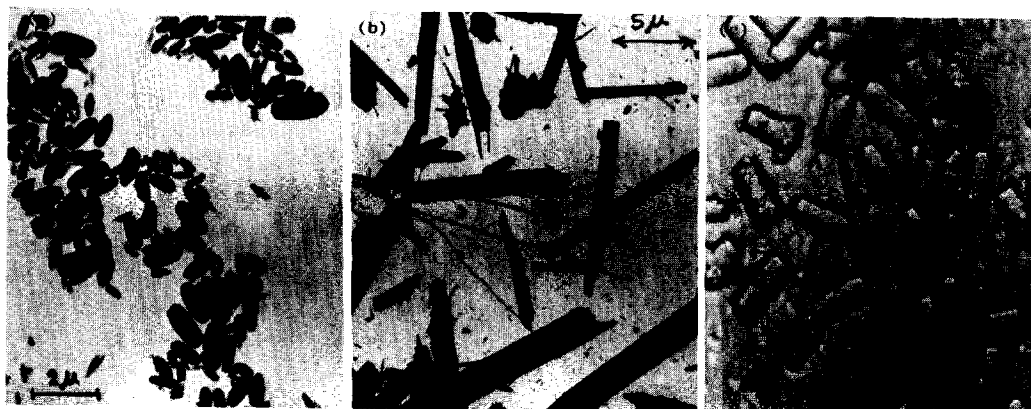
FIG. 5. Electron and light photomicrographs: (a) synthetic TMA offretite, (b) natural erionite, and (c) synthetic erionite.
